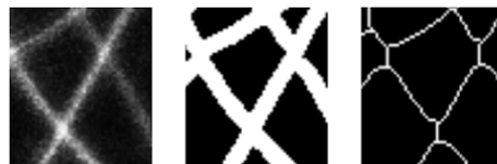
Fig. 1. From left to right: original image, binary segmentation, skeletonization. After skeletonization, some junction points turn into more than one junction, which creates many false, short filaments.
